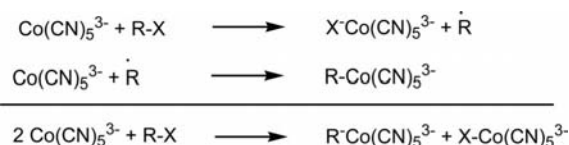
Scheme 5. Mechanism of the one-electron oxidative addition of alkyl halides to [\text{Co}(\text{CN})_5]^{3-} . [19]
